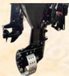
Steel Safety Cover Around The Propeller of OBM
